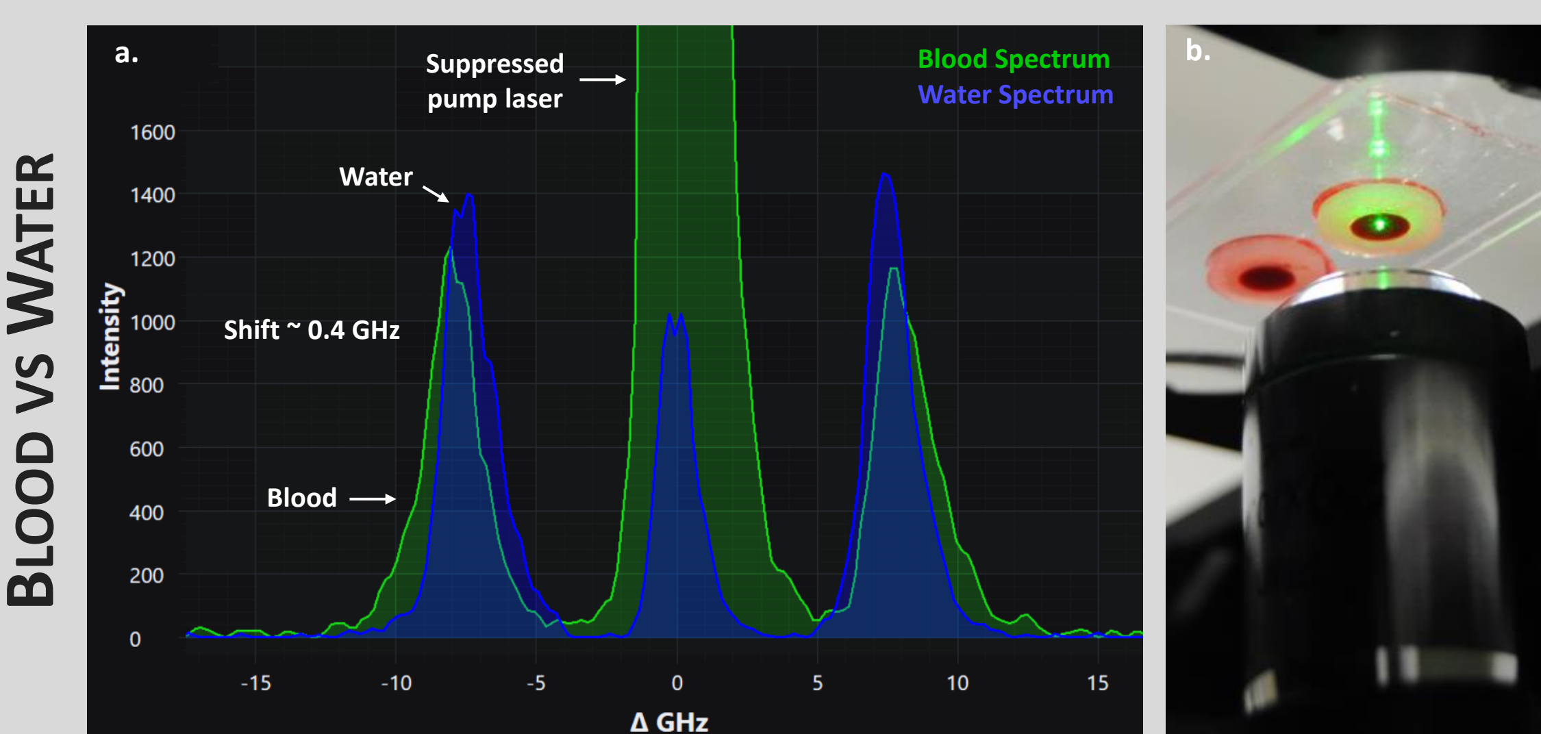
a. Brillouin spectra of blood (green) and water (blue). Brillouin frequency shift between water and blood ~ 0.4 GHz. 15 mW at 532 nm, blood spectrum: 1 sec (avg x10), water spectrum: 200 msec (avg x10). b. Excitation configuration showing blood wells.
